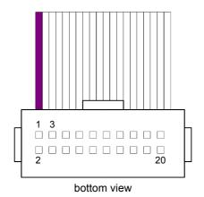
1 - 4:  $V_{cc}$  (4.5 - 5.5 V dc stabilized, 2 A)
