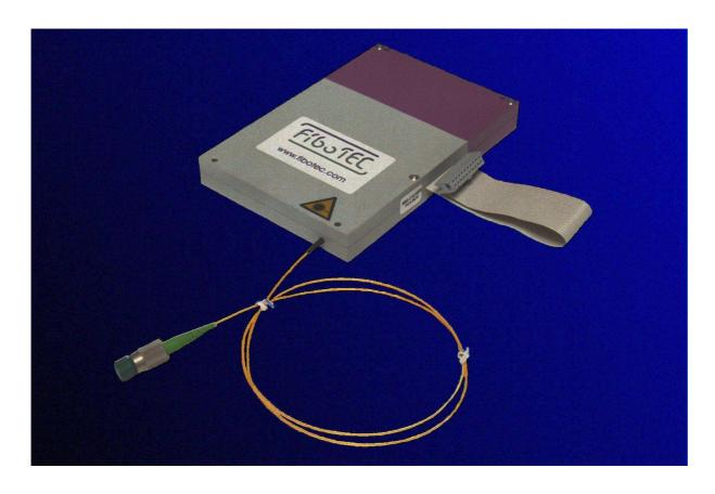
The Broadband Source "BBS CL 17P3 FCA M02" is a power-stabilized C+L-band ASE light source emitting a continuous spectrum in the wavelength range 1520-1610 nm. The ASE emission is achieved by optically pumping an erbium-doped fiber with a semiconductor laser of 980nm pump wavelength. The ASE output power exceeds 17dBm, emitted from a single-mode fiber with FC/APC output connector.
